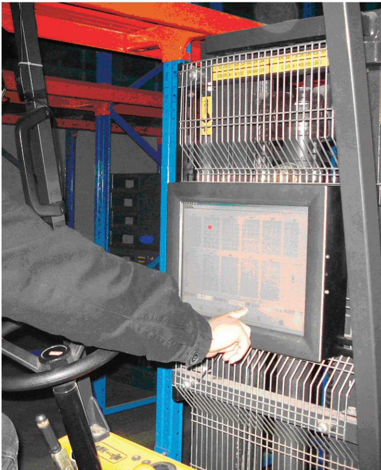
Figure 7. A touch screen computer fixed on forklift.
